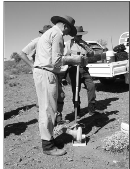
Using the Niton portable XRF analyser at Broken Hill
