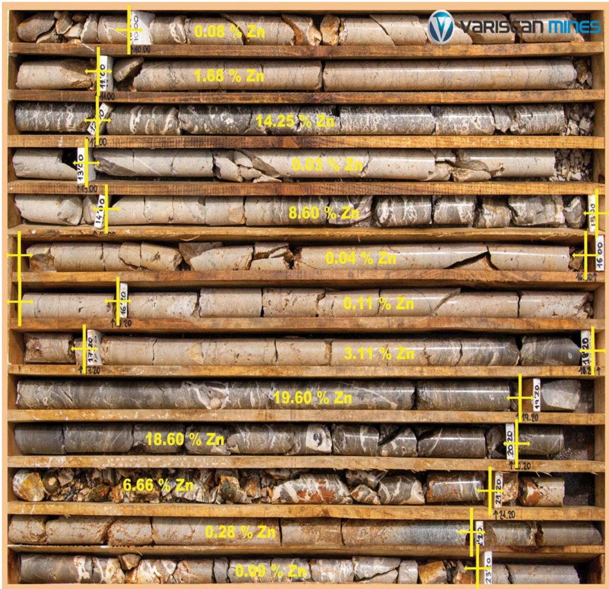
Figure 5. Diamond Drill Core from NOVDD058 in SW Zone illustrating massive sphalerite in dolostone
