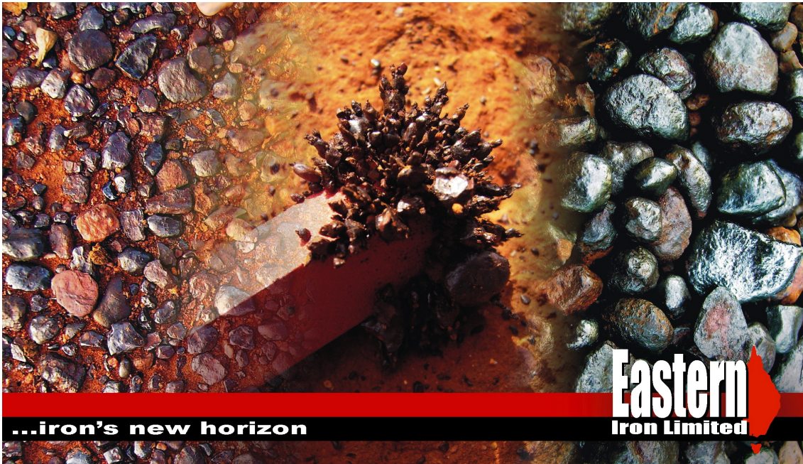
Figure 1 Material in iron-rich palaeochannels has been confirmed as maghemite ( \text{Fe}_2\text{O}_3 ). Simple “bench scale” beneficiation test work confirms that gravel from channel fill material with a bulk grade of 10 to 30% Fe (left) can be beneficiated to >50% Fe using magnetic separation to produce a lump sized product (right).
