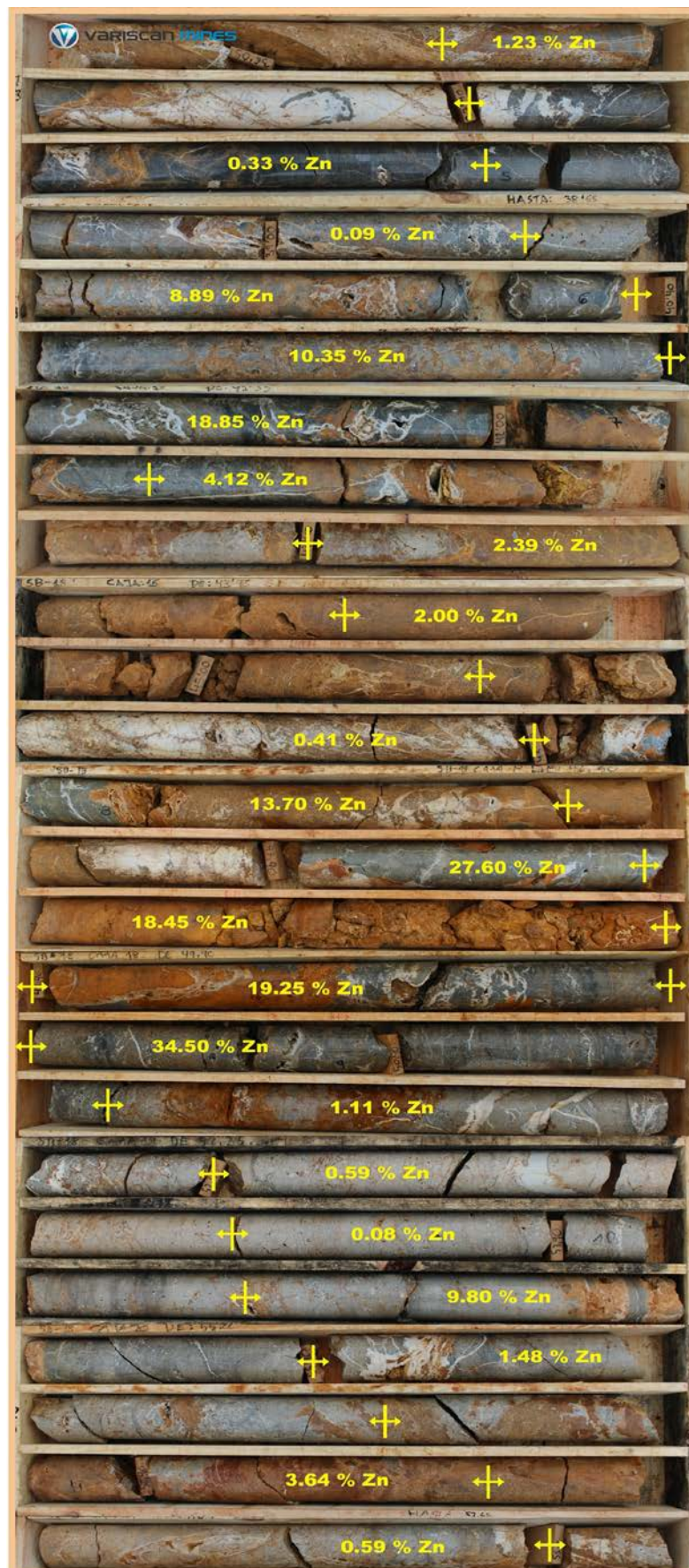
Figure 4. Photograph of mineralised core intervals from drill hole SB-18, with overlain zinc assay results. (Hole depth shown from 36.4m to 58.4m)
