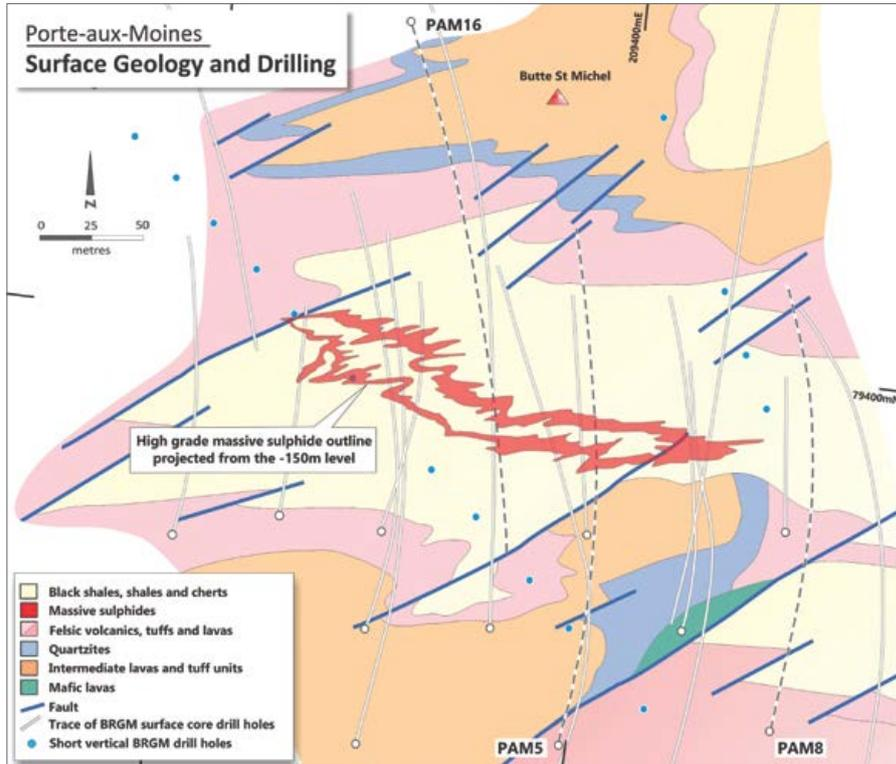
Plan view of the surface geology at Porte-aux-Moines and BRGM core drilling showing the location of PAM5, PAM8 and PAM16 with the approximate projected position of the high grade massive sulphide zones 150 metres below the surface as interpreted by the BRGM.
