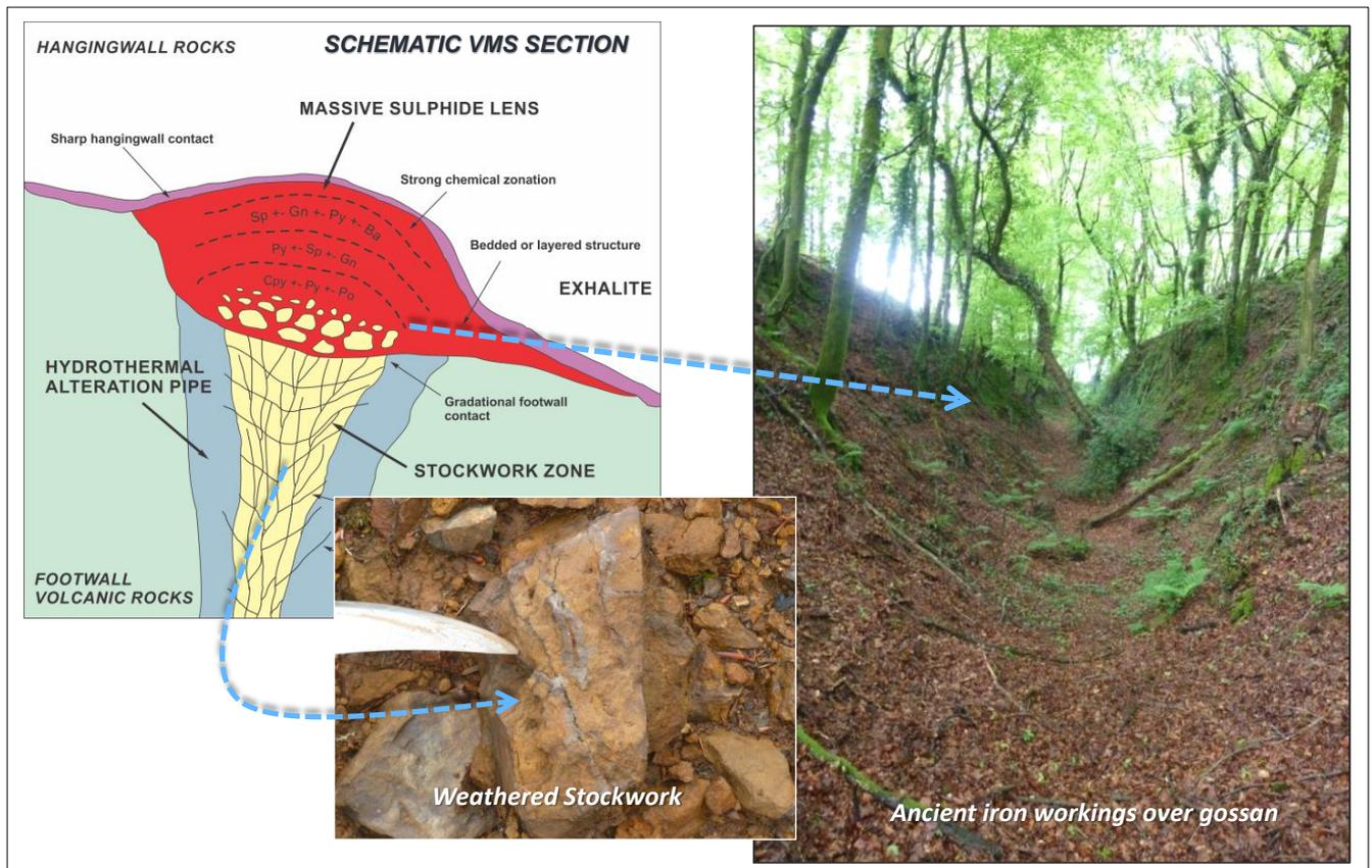
**Figure 4 – Photos from the old iron workings within the Merléac PER showing the interpreted relationships of the weathered, iron-rich material to the VMS deposit model as outlined by the USGS**
