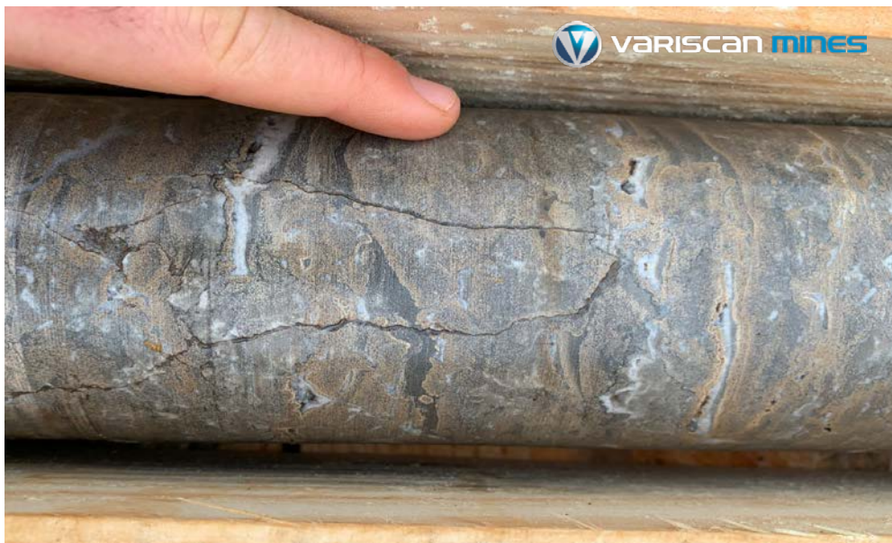
Figure 1. Richly mineralised (sphalerite) drillcore from Drillhole SB-18 step-out from the San Jose Mine (refer note 1 )
