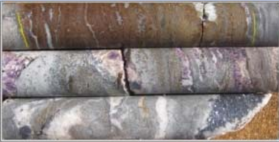
Core from Hole DF2 shows massive sphalerite, fluorite and galena
